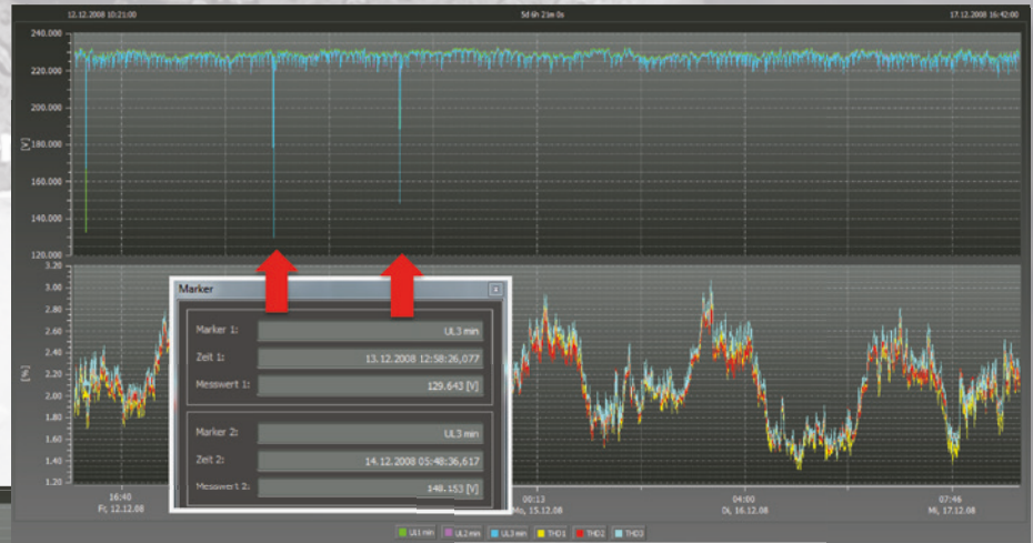
Extreme-values of voltage and current in millisecond-timestamps
