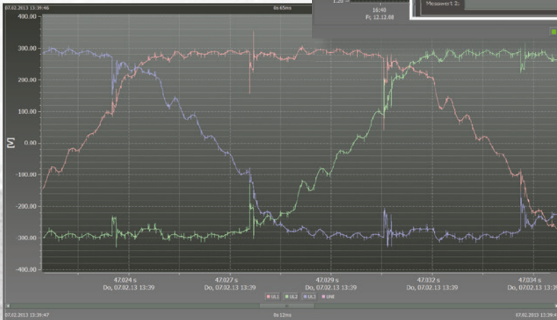
Oscilloscope recorder – Extremely high resolution due to 24 Bit A/D converters at the input of all voltage and current channels
